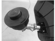
To remove the cutting head, put a locking tool in the hole of the shaft. Then unscrew the cutting head. This will have to be done tool off and cooled.
