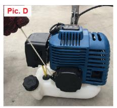
5). After the machine has started, return the choke to the ON position
